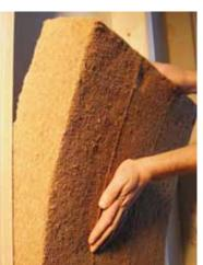
As with all STEICO natural fibre insulating materials, STEICOflex is particularly user friendly and will not knowingly cause itching or scratching – whether during cutting or installing. In order to make simple and uncomplicated cuts, it is best to use a special STEICO insulation knife or an electric all purpose saw (recommendation: Bosch GFZ A 14-35). Custom made insulation knives available direct from STEICO.
