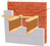
Minimum 38 \* 38 perimeter noggin skew nailed or fixed to joist using propriety clip. Noggin to be fixed 25 - 75 mm from face of wall
