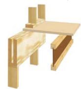
Blocking may overhang the inside face of the wall by half the blocking width
