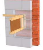
Restraint straps may be required for buildings over 2 storeys or where joists have less than 90 mm of bearing. Please consult hanger manufacturers literature for further information
