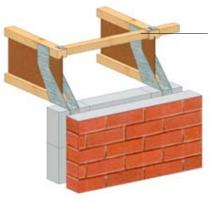
Minimum 38 \* 38 perimeter noggin skew nailed or fixed to joist using proprietry clip. Noggin to be fixed 25 - 75 mm from face of wall
