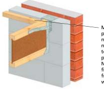
Minimum 38 \* 38 perimeter noggin skew nailed or fixed to joist using proprietry clip. Noggin to be fixed 25 - 75 mm from face of wall
