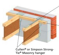
Restraint Straps fitted as manufactureres details
