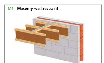
Galvanised masonry restraint strap fixed to minimum 3 joists in accordance with manufacturers recommendations. Blocking may be full depth I-joists or solid timber. Where solid timber is used ensure the size is a minimum of 38 mm x half the joist depth. Do not notch the flanges.
