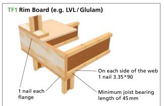
Minimum nailing for class 1 structures to be 3.00\*75 nails at 300 mm centres which should be applied at each interface where lateral loads are to be transferred. Refer to UKTFA "Design Guidance on Disproportionate Collapse" for further information
