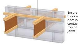
blockwork does not contact the top of the joists
