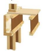
Blocking may overhang the inside face of the wall by half the blocking
